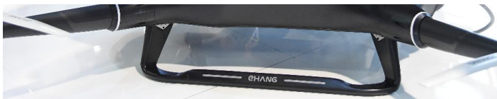
LAS VEGAS, NV – JANUARY 07: An EHang 184 autonomous-flight drone that can fly a person is displayed at CES 2016. The 18-foot-long, 440-pound drone can fly up to 63 mph for 23 minutes and go about 20 miles. It can carry one passenger who does not need to pilot the drone. Once a destination is entered, only a take off or land button needs to be pushed to travel. (Photo by Ethan Miller/Getty Images)
